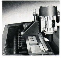
\*Built In Grinder A further aid to productivity. Cutters can be ground without removing them from the machine - saving "down-time". Encourages regular sharpening of knives.
