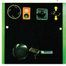
Power Rise and Fall Rise and fall switch with fine adjustment. And digital read-out for ease of operation and repeatable accuracy.
