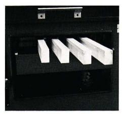
\*Sectional Feed Rolls High productivity with multiple feeding of timber of uneven thickness.
